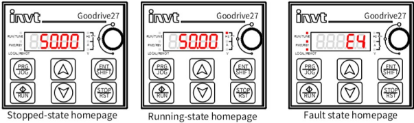
Figure 5-2 Status interface display
